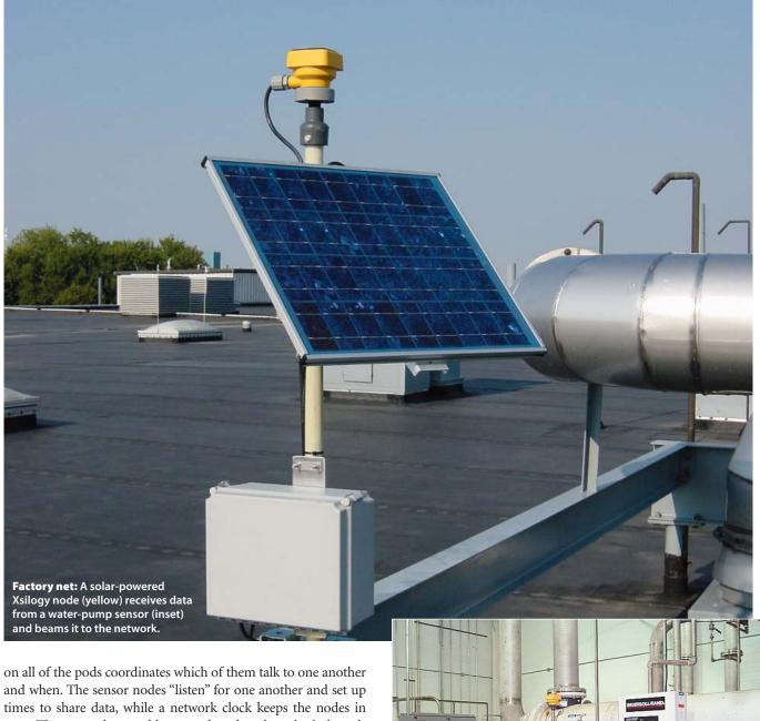
on all of the pods coordinates which of them talk to one another and when. The sensor nodes "listen" for one another and set up times to share data, while a network clock keeps the nodes in sync. The network resembles a mesh rather than the hub-and-spoke arrangement used for cell phones; instead of linking each sensor directly to a central communication point, the nodes send data only to neighbors within radio range, saving power.
